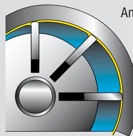
An oil film on the stator is inside surface and prevents wearing of the moving parts, avoiding a direct contact between the stator itself and the blades.
